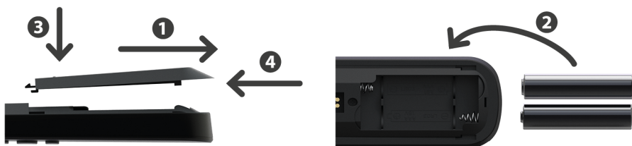
Figure 2: Inserting the batteries
