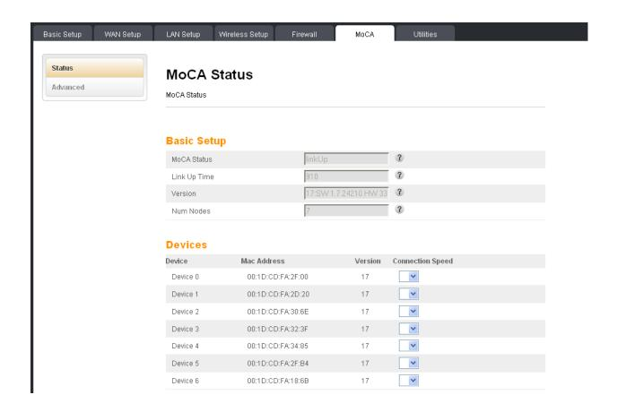
Unless using a wired Ethernet connection, the Moxi Gateway communicates with the Moxi Players using Multimedia over Coax Alliance (MoCA) over the home coax network. All MoCA traffic is between the Moxi Gateway and up to six Moxi Players.
